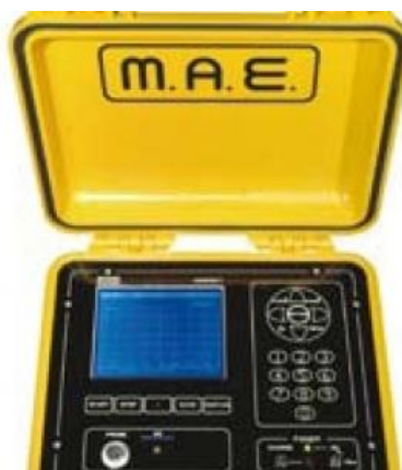
Figure 1. Device for measuring thermal conductivity in situ.
